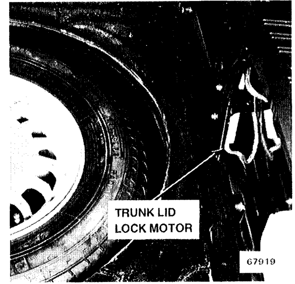
Figure 5 - Middle Rear Of Trunk
